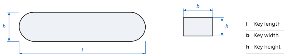
Parallel Key Form A DIN 6885A - dimensions
